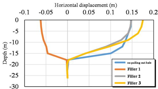
Fig. 8 Graph comparing the horizontal displacements of the ground centre line
