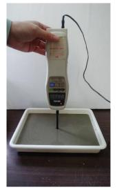
Fig.4 Simple penetration test
